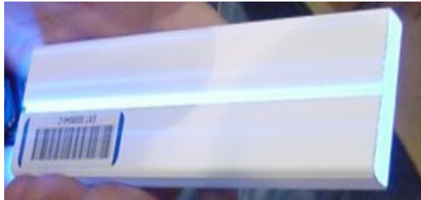
Extruded polystyrene doped with fluors, 14 pe per passing muon
